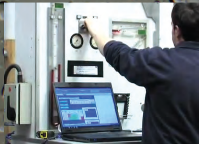
'Laboratory' tests for water ingress, wind resistance and air permeability
